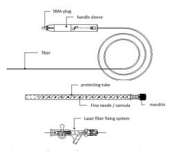
When using fine needles, correct inner diameters have to be chosen.
